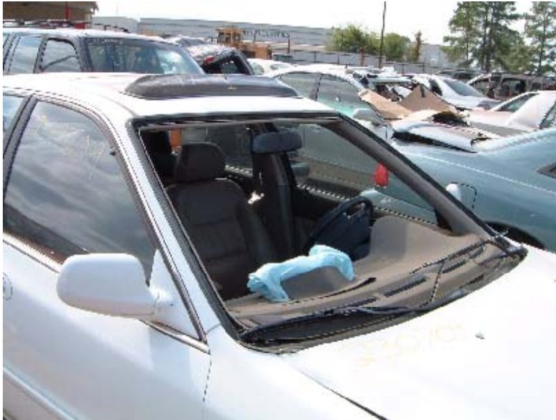
Exhibit F – FMVSS 208 and 212 failure-frontal crash with a blown out windshield
